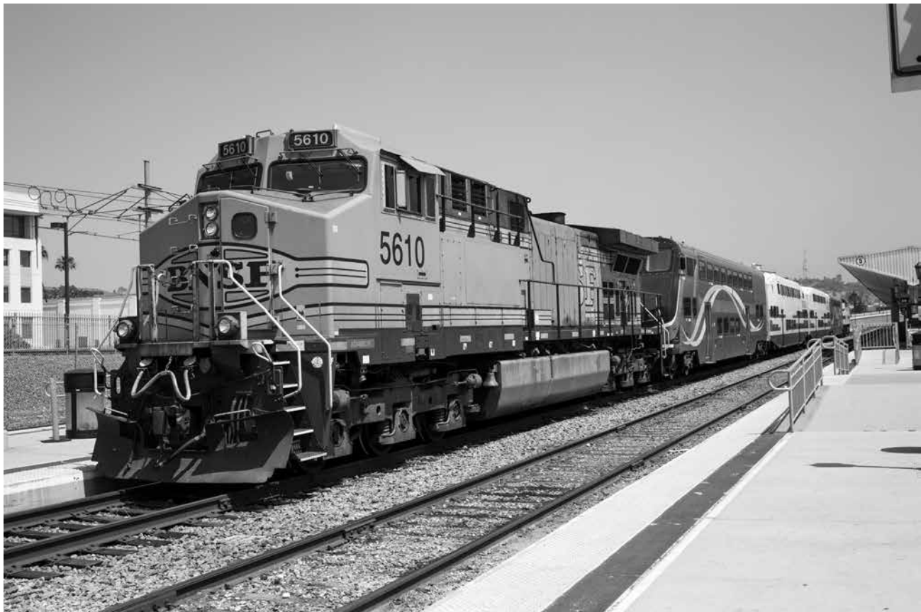
This Metrolink train, seen at Los Angeles Union Station, represents a sight no longer seen in the SCV. The leased BNSF locomotive is coupled in front of the train's Hyundai-Rotem cab car after one such car derailed in 2015 after hitting a pickup truck in Oxnard. The cab cars' front ends have since been strengthened, so the BNSF locomotives have been returned to that railroad.
