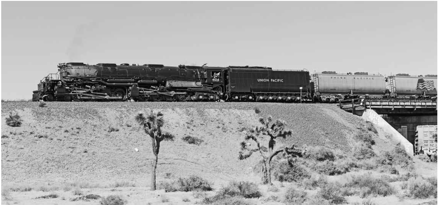
The world's largest steam locomotive revisited Southern California this October. Union Pacific 4014, a 4-8-8-4 "Big Boy", had been on display for many years at the Los Angeles County Fairgrounds in Pomona. It was returned to service by the railroad after a 5-year restoration in Cheyenne, WY. It is seen here approaching Cajon Pass on October 9, before leading a Colton - Barstow excursion the following weekend.
